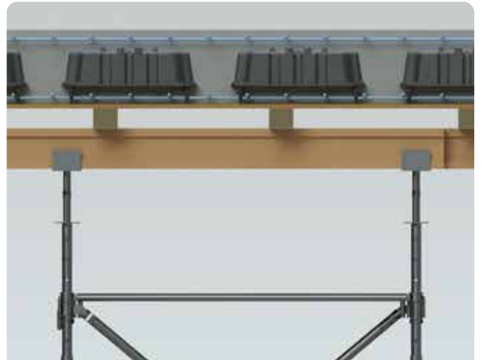
6. Finish casting in a second phase, when the concrete is slightly plasticized or when the units are fixed in concrete. Level the surface as per requirement.
